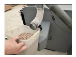
After filling the screw, empty the pot and then run the pellet feeding screw for 15 minutes.
