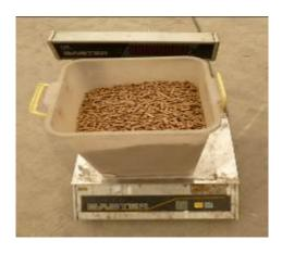
Weight the pellets in pot. Note the weighted pellets in grams. (X = ..... gram)
